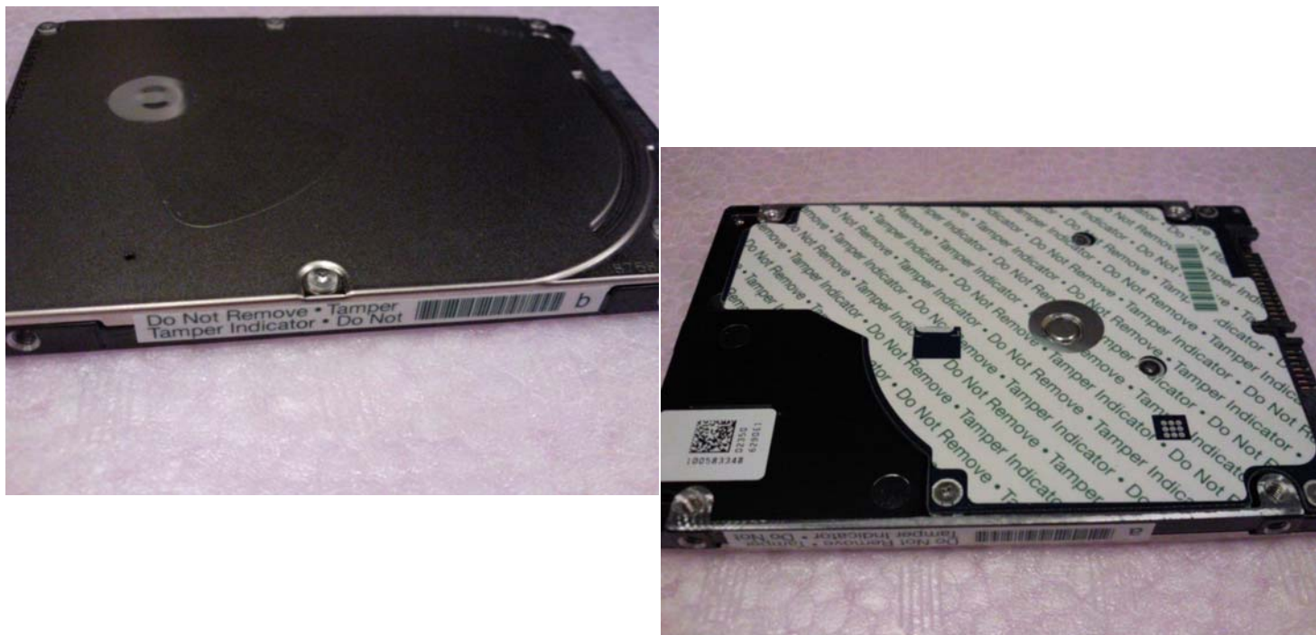
Figure 4 Example of FIPS tamper evidence labels.
