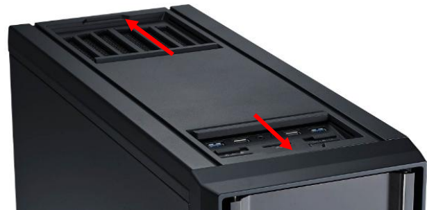
Sliding covers protect the I/O and top vent from dust
