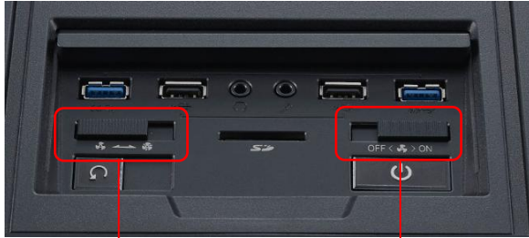
Fan controller (Front: 2, rear: 1)
