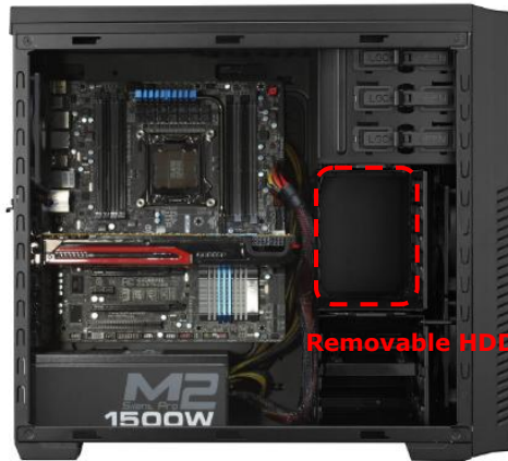
Supports all high-end graphics cards with the 1 st HDD cage removed
