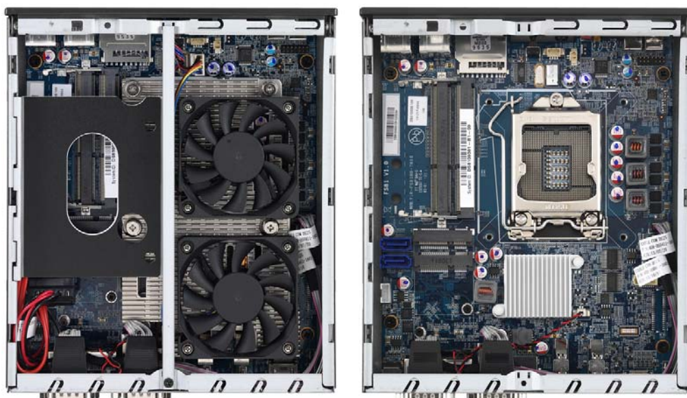
Top view without chassis cover (with and without drive tray and cooling system)
