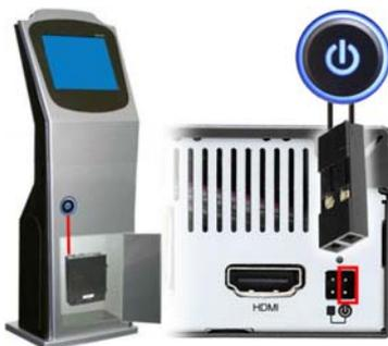
**External power button by separate remote line**
