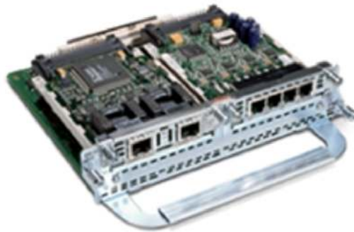
Figure 1. NM-HD-2VE with one VWIC-2MFT and one VIC-4FXS/DID
